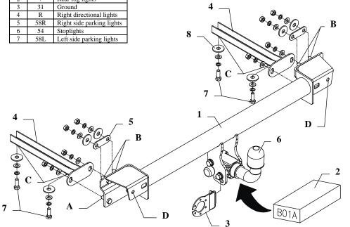
This towing hitch is designed to assembly in following cars: BMW 3 Series E30, 4 door, Coupe, produced since 10.1982 till 09.1990, BMW 3 Series E30, Estate, except M Package, produced since 09.1987 till 08.1994, catalogue no. B01A and is prepared to tow trailers max total weight 1400 kg and max vertical load 75 kg.
